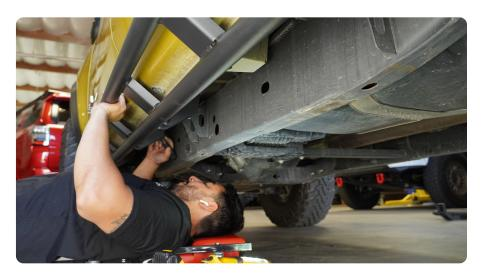
STEP 4 | Adjust the slider side to side to your preferences. For this installation we adjusted the slider all fully forward.
