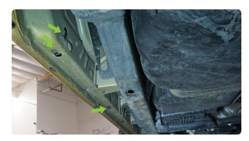
STEP 2 | If equipped, remove the (8) factory nut clips from the rocker panel using a trim tool or flathead screw driver to remove factory nut clips
