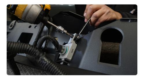
STEP 20 | Feed the factory main wiring harness through the bumper mounting brackets.
