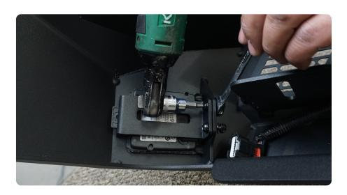
STEP 25 | Remove the 90 degree cable guide from the blind spot monitor wiring harness connector using a pick or small flathead screw driver to pry the cable guide off.
