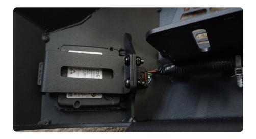
STEP 27 | Install the trailer hoist cover and trailer connector socket into the bumper by pressing each through the front of the bumper until each one is fully clicked in.
