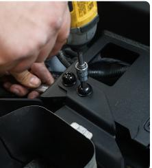
STEP 32 | With assistance mount the bumper on to the vehicle. Use a 18mm socket or wrench and the provided M12 hex bolts to loosely secure the bumper in place.
