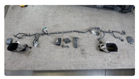
STEP 15 | The passenger side inner parking sensors wiring loom will need to be cut back to prevent the harness from pinching.
