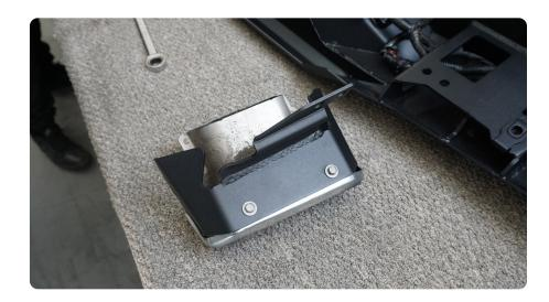
STEP 31 | Use the provided M12 Allen head hardware, an #8 Allen tool and 19mm wrench to mount the exhaust tips to the DV8 rear bumper.
