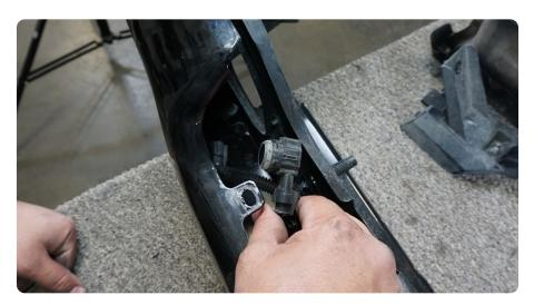
STEP 13 | Remove the sensor bezel by depressing the bezels locking tabs and pressing the bezel out through the front of the bumper.
