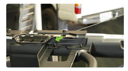
STEP 18 | Non-Raptor Hard Top Models: Remove (2) of the three factory bolts on each side that secures the hardtop Latch brackets using a T50 Torx bit.
