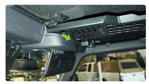
STEP 29 | Secure the M6 hardware at the front and rear of the molle panel using a #4 Allen tool and 10mm wrench.
