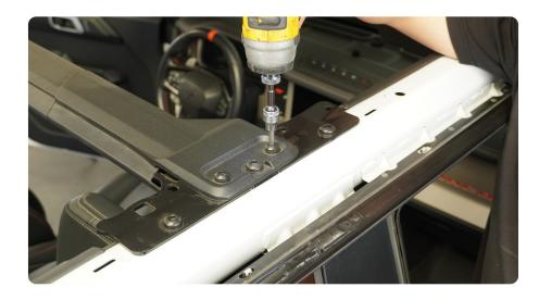
STEP 13 | Use a T50 torx tool to remove the rear factory bolt that secures the latch plate to the roll bar on both sides.
