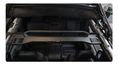
STEP 25 | Use a #4 Allen bit and 10mm wrench to secure the hardware holding the cross-brace to the roll bar mounting bracket.
