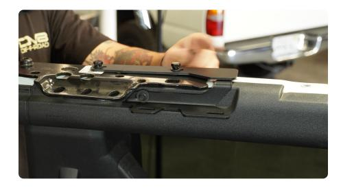
STEP 16 | (Bronco Raptor only) Place the DV8 cross bar under the roll bar brackets and secure the cross bar in place using the provided M6 hardware.
