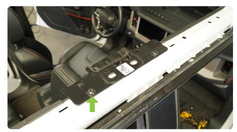
STEP 14 | Loosely Install the roll bar brackets using the factory hardware and an 8mm socket. Make sure the bracket grabs the slotted hole on top of the roll
