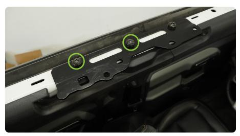
STEP 19 | Use a 8mm wrench to remove the bolt on the interior of the roll bar.
