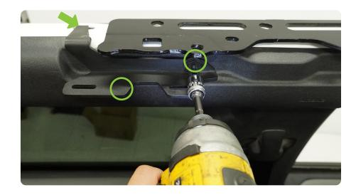
STEP 21 | Loosely install the provided pressure plate on top of the factory hardtop latch plate and DV8 roll bar bracket using the factory hardware and an T50 torx tool.
