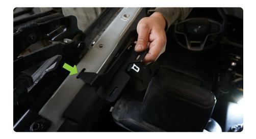
$\begin{array}{c|c} \text{STEP 23} & \text{Place the provided spacers} \\ \text{over the factory threaded holes on top of} \end{array}$ the roll bar.
