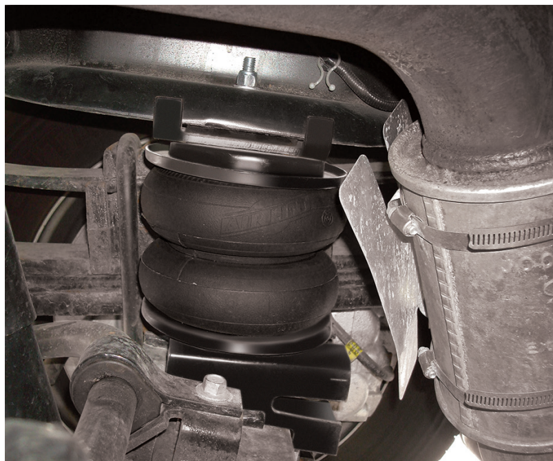
Inside, above axle view of passenger's (right) side installation.
