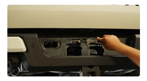
STEP 5 Using a pry tool, remove the (4) top panels along the top of the bumper. Take your time since these can be difficult.
