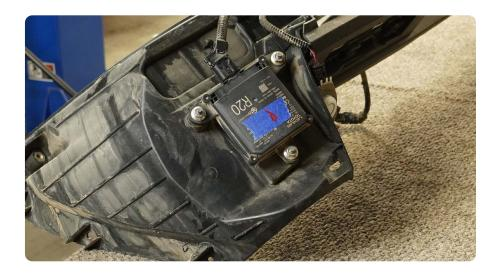
STEP 12 | Using a 10mm socket, remove the BSM from the bumper. Avoid unplugging from harness.
