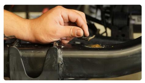
STEP 9 | Moving to the bumper, using the push pin pry tool, remove the outside caps of the bumper. These will need to be removed to access the blind spot sensors and harness.
