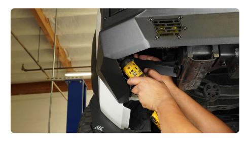
STEP 34 | Remove the 7-pin plug from the factory bumper and reinstall into the new DV8 bumper.
