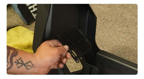
STEP 21 | Using the provided BSM spacers, (2) per side, mount the BSM using the same hardware holding the mesh.
