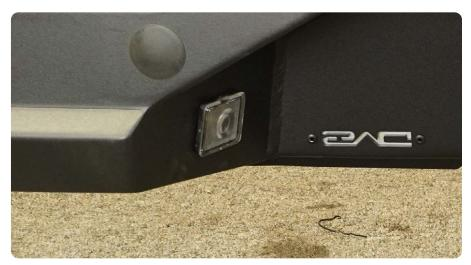
STEP 15 | Lay out the harness so the sensors line up with the new bumper. We are assembling this bumper upside down for ease since the factory was disassembled upside down as well.
