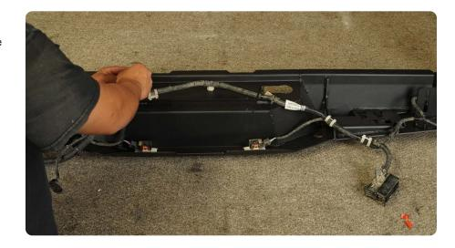
STEP 24 | Once all sensors are in place, using the provided zip tie tabs, secure the harness to the bumper so it does not get pinched during install.
