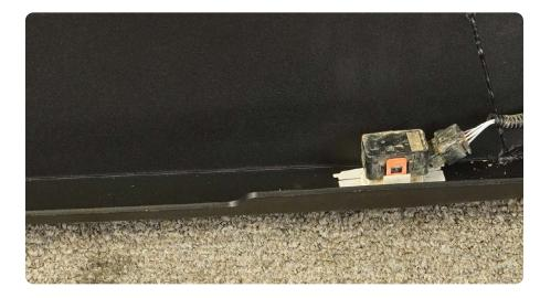
STEP 25 | optional: Install 3" lights onto the bumper using the hardware provided with the light.
