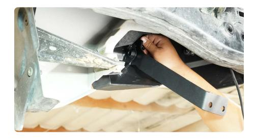
STEP 32 | Using the provided long (4) M12 bolts and nuts, secure the side support brackets to the frame.
