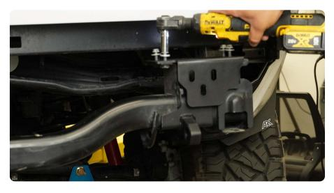
STEP 27 | With assistance, place the bumper onto the truck mounts. Using the provided M10 hardware, secure one bolt into place to hold the bumper to the mounts.
