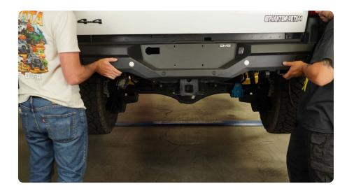
STEP 29 | With the bumper removed, tighten the mount bolts until secure using a 12mm socket/wrench.
