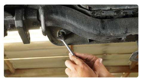
STEP 3 | Moving to the sides, using a 12mm socket, remove the bolts holding the side support brackets to the frame.
