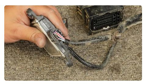
STEP 19 | For this install, we Plasti dipped the sensor lightly to cover the white lettering.
