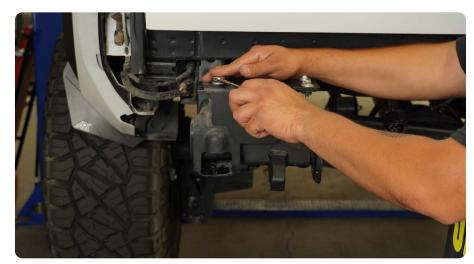
STEP 30 | Reinstall the bumper, and loosely secure using the provided (6) M10 bolts and a 16mm socket.
