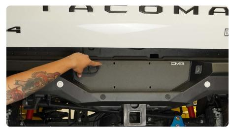
STEP 35 | Moving to the back of the bumper, replug the 7-pin connector and the main plug harness to the truck. Ensure all sensors and license plate light are reconnected firmly before turning on the truck.
