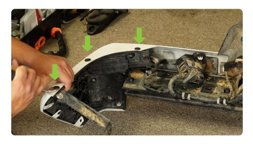
STEP 10 | With the clips removed and the cap loose, gently pry off the sensor AND sensor bezel from the inside of the cap.
