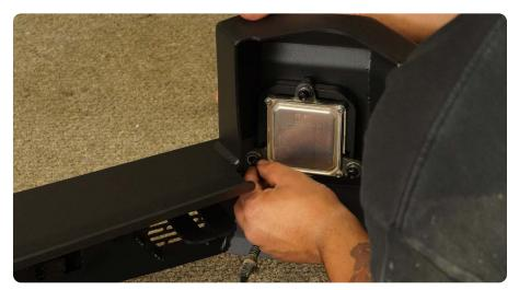
STEP 22 | To mount the inner sensors, remove the wired guide near the sensors similar to the BSM sensors.
