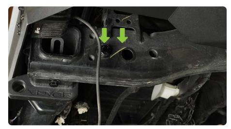
STEP 33 | Using a 18 and 19mm sockets, tighten the frame bolts and the bumper bolts to secure the support brackets in place.
