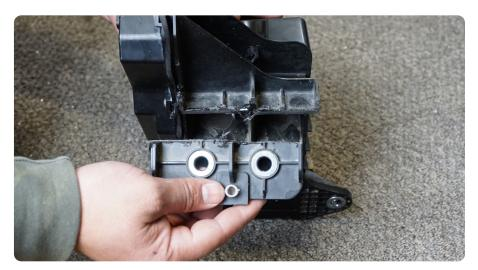
$\begin{array}{c|c} \text{STEP 41} & \text{Trim the small remaining} \\ \text{mounting tab off the motor as shown.} \end{array}$
