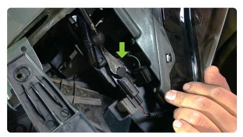
STEP 8 | Disconnect the wiring plugs located behind the grille on the passenger side of the vehicle underneath the grille's upper mounts.
