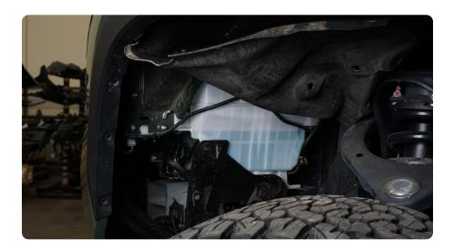
STEP 3 | Using firm pressure, pull the fender flare away from the truck to the side to release the clips.
