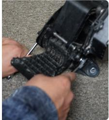
STEP 37 | Remove the black caps, the white plastic spacers and the spring from the inside, and set the arm off to the side.
