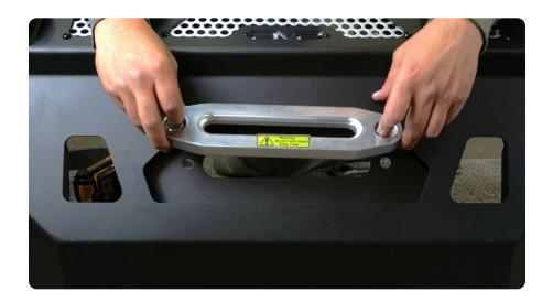
Install the winch plate using the provided M14 hardware and a 21mm and 19mm wrench.
