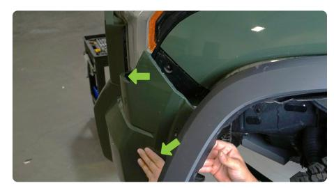
STEP 4 | Reach behind and underneath the bumper to remove the black plastic trim by pressing out the clips from the inside.
