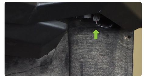
STEP 57 | Connect the wiring located on the passenger side of the vehicle underneath the upper mounting bracket on the grille. (From Step 8)
