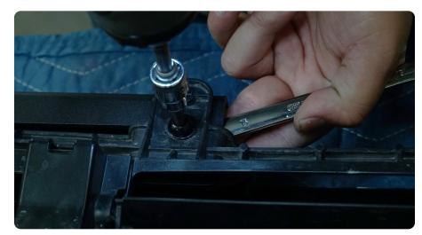
STEP 34 | Use a 10mm socket and the factory bolts to install the shutters.
