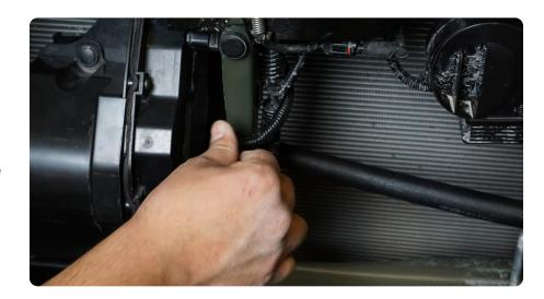
STEP 50 | Place the wiring harness into the bumper and run the wires so that the sensors are at their approximate location of install. Secure the wiring in a safe location.
