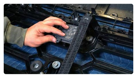
STEP 27 | Remove upper mounting bracket from the grille by pulling it away from the grille to release the clips.
