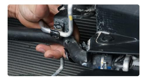
STEP 45 Use a 10mm socket to remove the bolt securing the vertical cross brace. Slip the cooling hose behind the cross brace and re-secure using the factory hardware.
