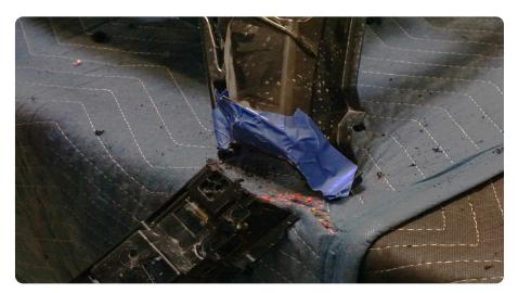
STEP 31 | Install the upper mount that mounts to the vehicle back onto the grille by clipping it back into place on the grille.
