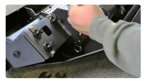
STEP 18 | If you are running pod lights, install them at this time using the hardware provided with the lights.
