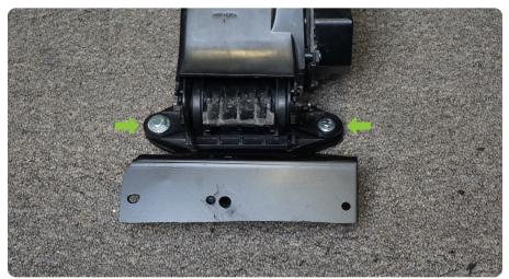
STEP 48 | Install the air dam bracket onto the horizontal cross brace using the provided M6 hardware and a 4mm allen bit. Connect the air dam motor wiring plug.
