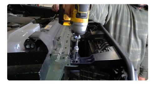
STEP 53 | Use the provided M6 hardware and a 4mm allen bit to secure the lower section of the grille to the bumper. The same tabs from step 36.
