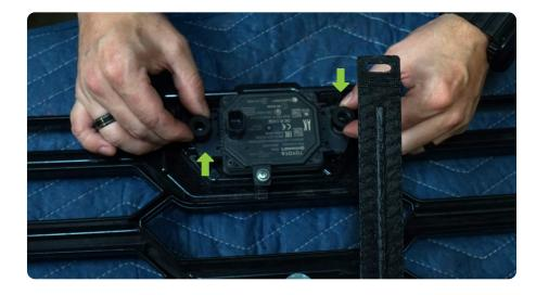
STEP 33 | Secure the shutters to the provided bracket using the provided M8 hardware with a 5mm allen bit and 13mm wrench.
