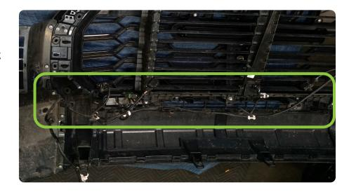
STEP 24 | Install the sensor plugs into the bumper.
