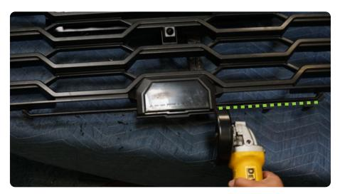
STEP 29 | Use an angle grinder to grind a small section off the bottom corners of the grille.
