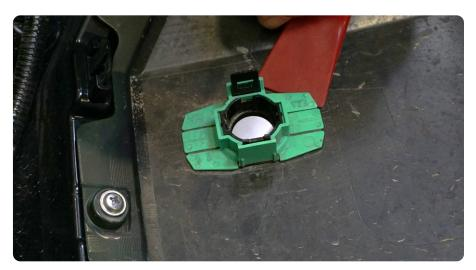
STEP 22 | Clean the residue off the sensor plug using a blade so that when installed, it will sit flush.
