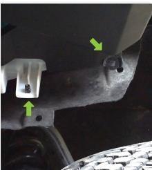
STEP 64 | Re-install the skid plate using the factory hardware and a 12mm socket. Double check all hardware is secure and that all wiring is connected.
