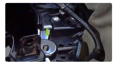
STEP 56 | Connect the wiring located behind the bumper in the fender well on both passenger and driver side of vehicle. (From Step 7)
