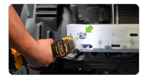
STEP 14 | Using the 14mm socket or wrench, remove the three nuts located on both sides of the crash bar. Remove crash bar and set off to the side since this will not be reused.
