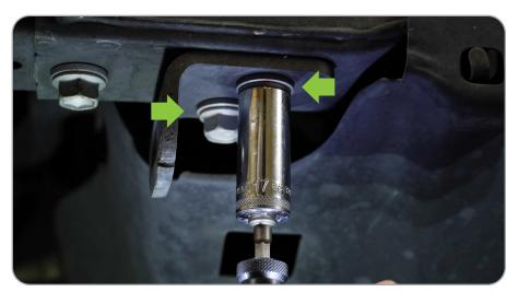
STEP 18 | Using the 17mm socket, remove the remaining bolt on the underside of the front frame crossmember to remove the frame extension. Repeat on opposite side.
