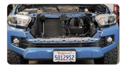
STEP 5 Using push pin removal tool, remove the four push pins securing the bumper to the vehicle.
