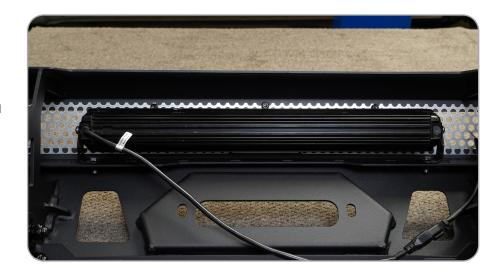
STEP 25 | If running 3" Pod lights on the wings, install them using the hardware provided with the lights.
