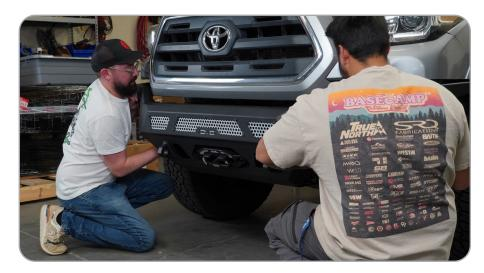
STEP 28 | Center the bumper on the vehicle, ensuring the ends of the wings are at equal distances and heights from the headlights are equal. Use a 14mm socket to secure the bumper in place.
