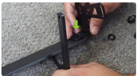
STEP 9 | Install the light bar to the mounting bracket using the hardware that was provided with the light.
