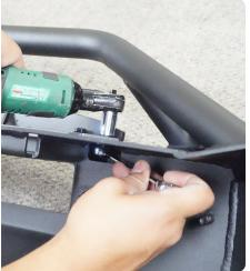
STEP 7 If you are installing a winch, mount the winch to the bumper winch plate at this time using the hardware provided with the your chosen winch.
