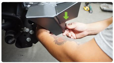
STEP 12 | Ensure the (6) main bumper stud nuts are torqued to 60ft lbs. Double check fitment and all hardware is secure.
