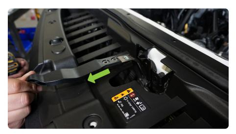
STEP 3 | Using a trim pry tool, remove all (10) valance retaining clips.
