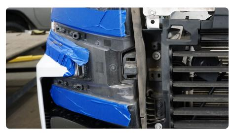
STEP 8 | Use an 18mm socket to remove the top two bolts on the bumper support bracket, for each side of the bumper.
