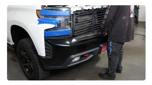
STEP 11 | Use an 18mm socket to remove the hardware securing the bumper mounting plate to the frame horns, and set it off to the side.
