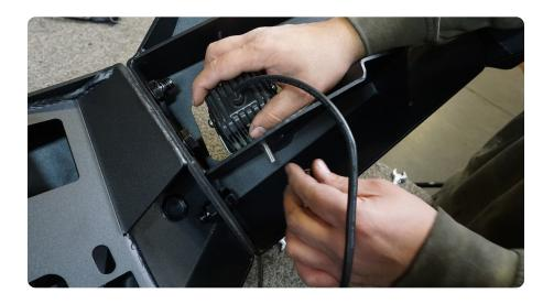
STEP 20 | Install the provided M12 nut clips by pressing them into place.
