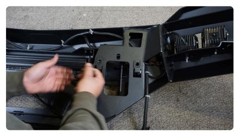
STEP 21 | Install the sensor bezels in the locations and orientation they were removed from the factory bumper.
