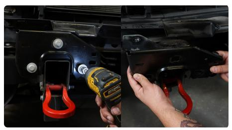
STEP 12 | Usean18mmsocket/wrench to remove the hardware securing the tow hook and set it off to the side.
