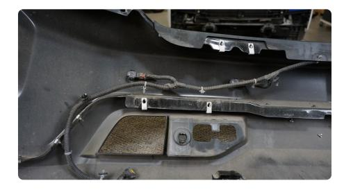
STEP 15 | Remove the sensors from the bezels by gently spreading the locking tabs to release the sensor from the bezel.
