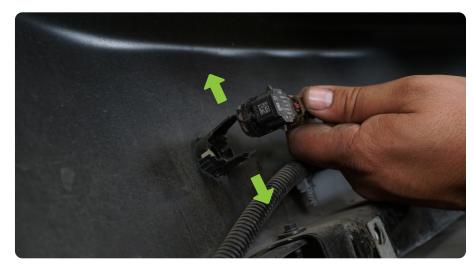
STEP 16 Use a pick or similar to carefully press the retaining tabs around the sensor bezel to gently push it out of the front of the bumper.
