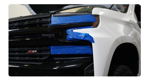
STEP 1 Use a trim clip tool to remove the fasteners securing the upper valance to the grille.
