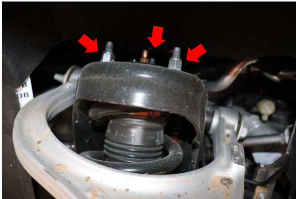
9. Remove three 18mm top hat nuts.
