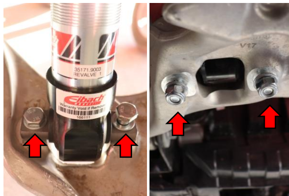
14. Use 19mm to install and tighten lower shock mount nuts and bolts to manufacturer specification.
