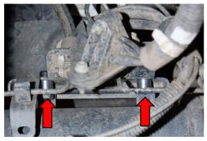
Remove the bolt from the driver side brake line bracket and install the provided bolt and brake line bracket spacer. Torque to factory specifications.
