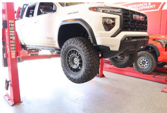
Step 2. Remove front tire using 21mm.
