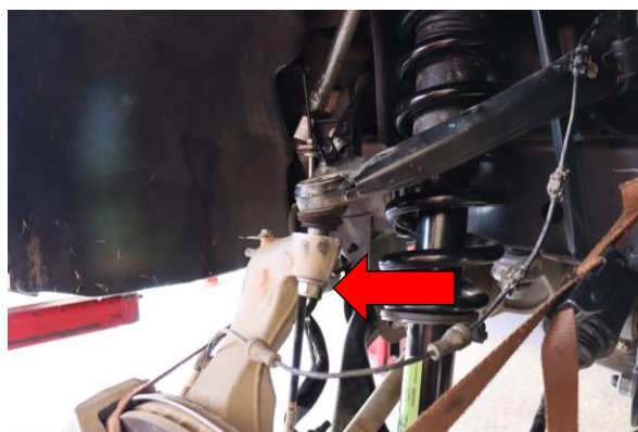
Step 6. Use an 18mm to loosen the upper ball joint nut. DO NOT remove it at this time.
