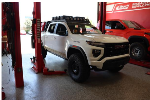
Step1. Lift and support vehicle.
