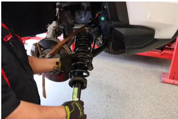
Step 11. Remove the shock assembly from the vehicle.
