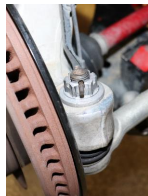
22. Install outer tie rod and upper ball joint cotter pins.
