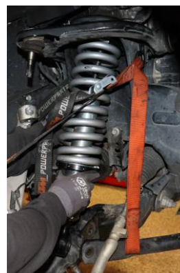
16. Install the PRO-TRUCK coilover by inserting up through the upper control arm.
