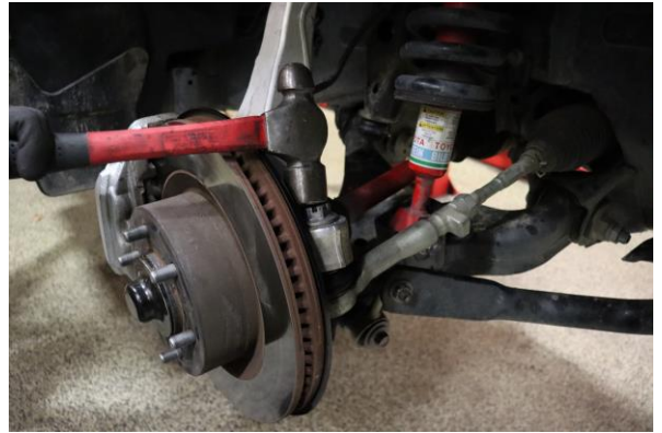
8. Use a hammer to remove the outer tie rod from the steering knuckle.
