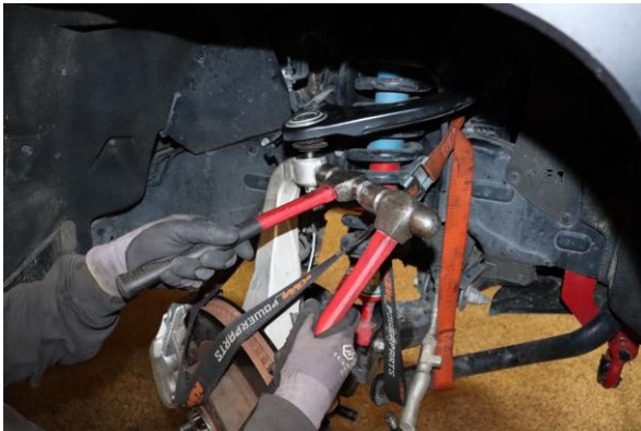
9. Use a hammer to knock loose the upper ball joint.
