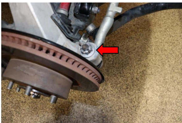
21. Install outer tie rod end in steering knuckle. Tighten to manufacturer specification.
