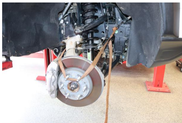
Step 4. Use a strap to prevent over extension of the axle during shock removal and installation.
