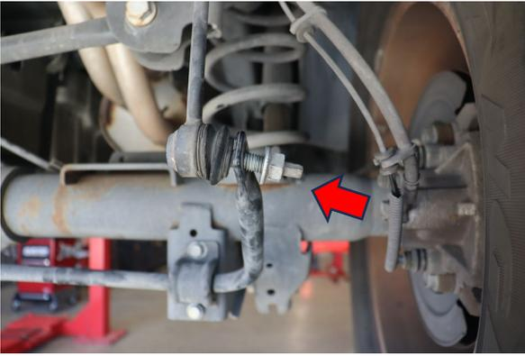
Loosen and remove OE rear end links from OE sway bar
