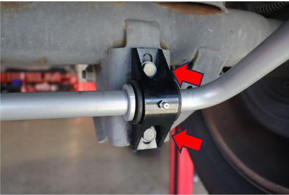
Install new bushings and brackets onto Eibach sway bar.
