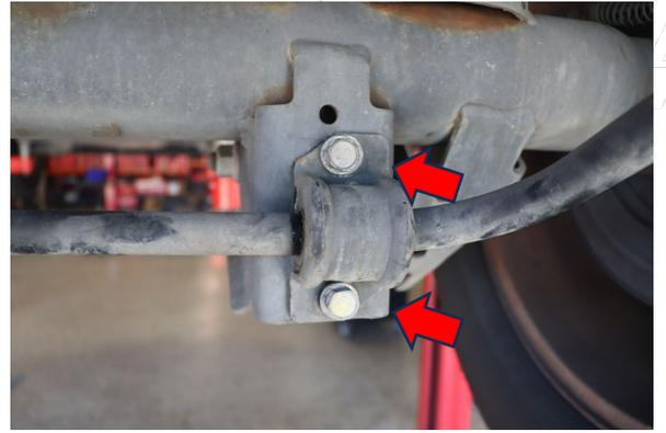
Loosen and remove OE sway bar brackets and remove sway bar.
