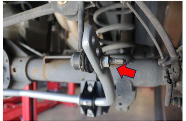
Attach factory end links to Eibach sway bar.
