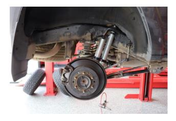
The reservoir should be mounted towards the top and pointing towards the axle on both sides of the vehicle. (Right Side pictured)
