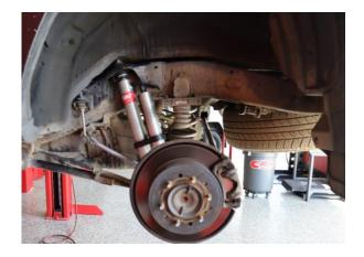
The Left and right shocks will have a different locating tab to orient the reservoir away from the frame. The locating tabs will be marked with a "L" or "R" to notate with side they belong on. The part number stamped on the shocks will also be marked. Failure to put the shocks on the correct side will cause issues fitting them to the vehicle and damage to your shock. (Left Side pictured)
