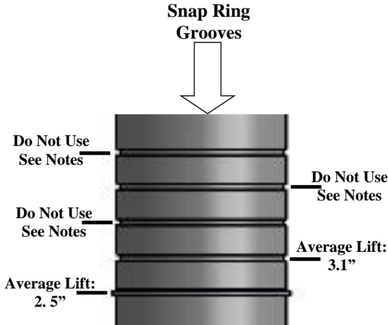
**Important:** Ensure that the snap ring is fully seated in the snap ring groove (you should be able to rotate the snap ring manually/by hand). **Note: Improper installation will cause permanent damage to the shock. Please refer to the Pro Truck Sport Damper instructions for more info regarding proper installation and fitment.**
