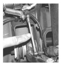
18. Clamp the OE ride-height sensors in a vice and gently twist the plastic ball socket ends off using a pair of pliers at the base of the socket. Be careful not to damage the plastic sockets. (See previous photo)
