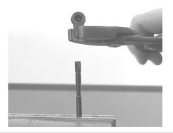
Locate the new Eibach ride height sensor links (Short Links) and thread one ball socket onto each end. Screw the sockets down until they gently bottom out.
