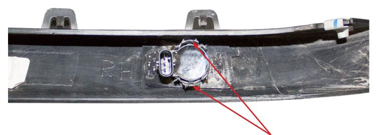
Release the parking sensor by spreading these two tabs
