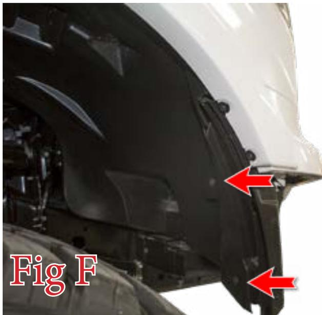
9. Pull the fender flare free from the valance. Then, pull the valance free to expose the air dam sitting behind it. (Fig G)
