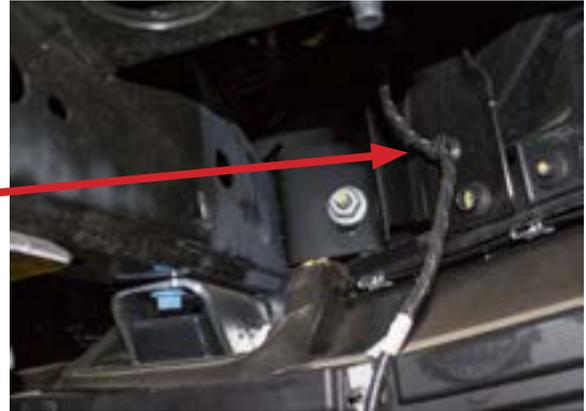
3. Using a 21mm Socket, remove the OEM bumper mounting bolts. There are two (per side) on the front side of the bumper and one (per side) on the rear side of the bumper. (Fig C)
