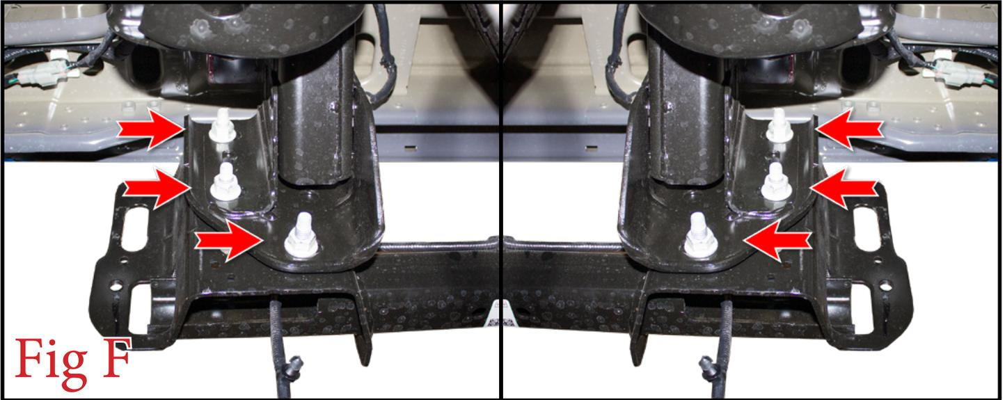
11. Pull the hitch down as low as it can go, then re-tighten the bolts from Step 10.
