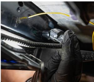
2.3 - Once the new fog light is installed, you will notice an extra yellow wire with a single connector. This wire connects to the additional harness that sits between the headlight and the vehicle's turn signal connection.
