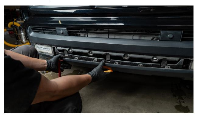
1.5 - Now, remove the screws at the back, and the shroud should come off completely.
