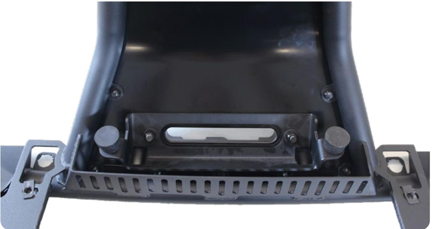
24. Set the bumper in place on the vehicle. Install the supplied 3/8" Bolts (x4) and 3/8" Fender Washers (x4) from the back side of the vehicle's frame horns (**They are located on each side of the frame**) "Fig S"
