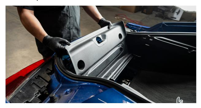
1.5 - With the center trim piece removed, you'll now have access to the clip securing the outer trunk liners. Carefully release these clips from both sides.
