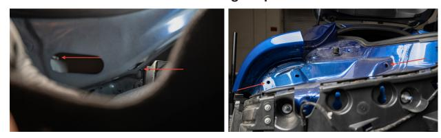
1.17 - With the tail light loosened, carefully pull it away from the vehicle. Disconnect the single connector and release the clip securing the wiring at the bottom of the light.
