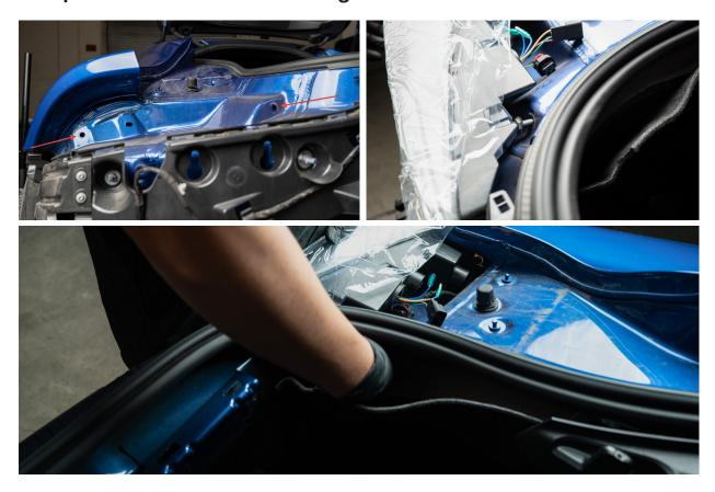
2.2 - With the tail light secured, connect it to the vehicle by inserting the provided converter between the vehicle's connector and the tail light connector.
