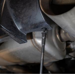
1.10 - Once the bolts are removed, there will be six clips that need to be released to fully detach the bumper. Use a flathead screwdriver to push up on the center of each clip while gently pulling the bumper to release them.
