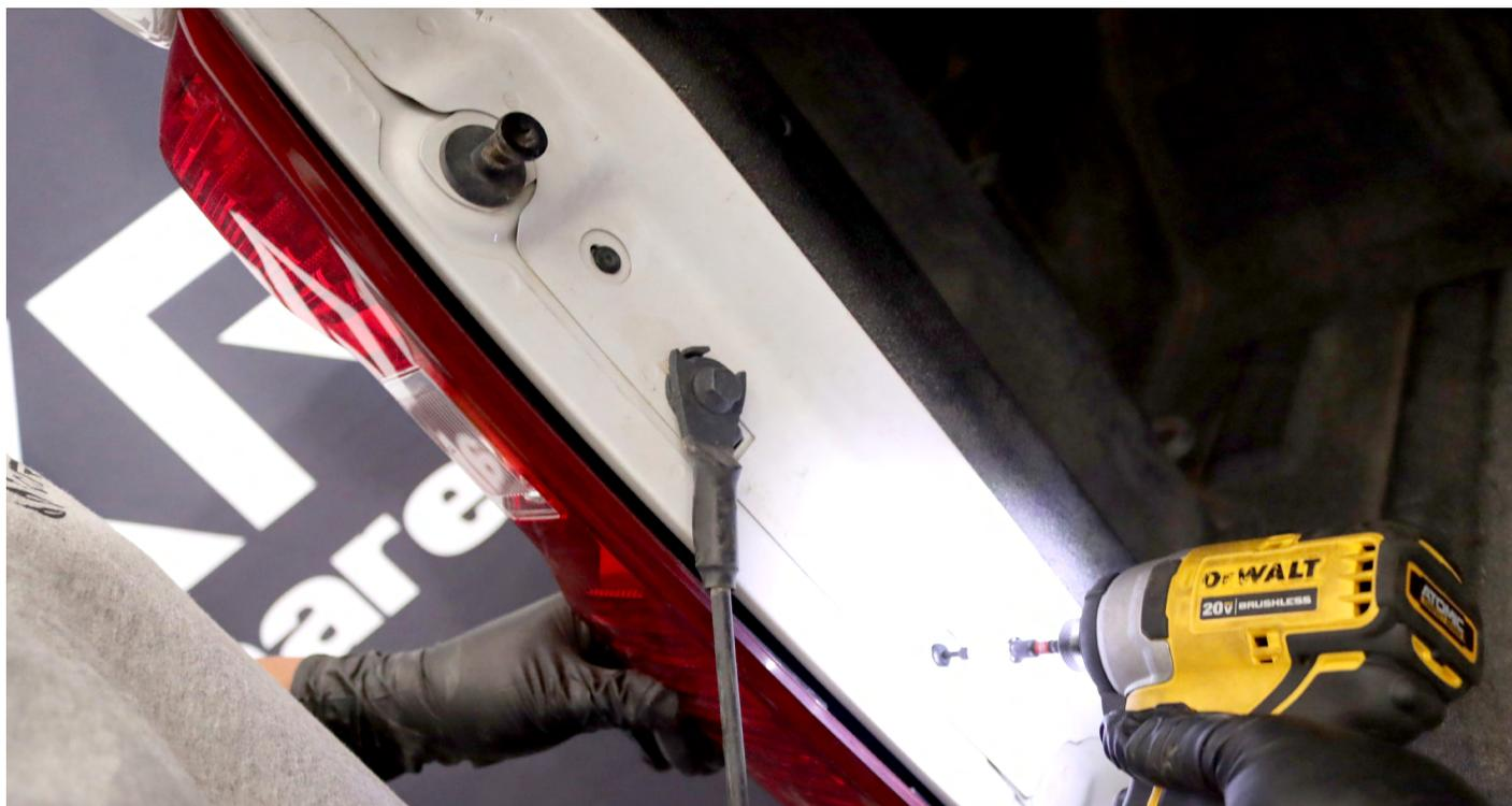
Remove the top and bottom T15 screws from each side of the tail lights.
