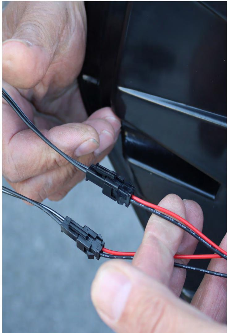
Plug the new ALPHAREX tail lights' connectors into the sockets. **DO NOT USE DIELECTRIC GREASE!**
