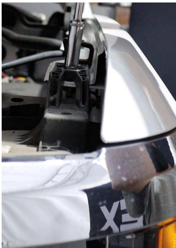
To access the headlight bolt from the inner bumper, first, remove the 2 X T15 screws from the wheelwell.
