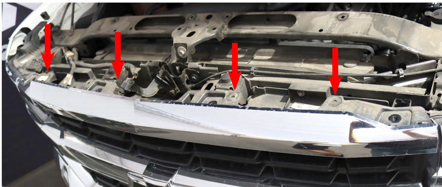
Subsequently, carefully pull the grille towards you to release it from the 6 insert mounts. Set it aside for later reinstallation.
