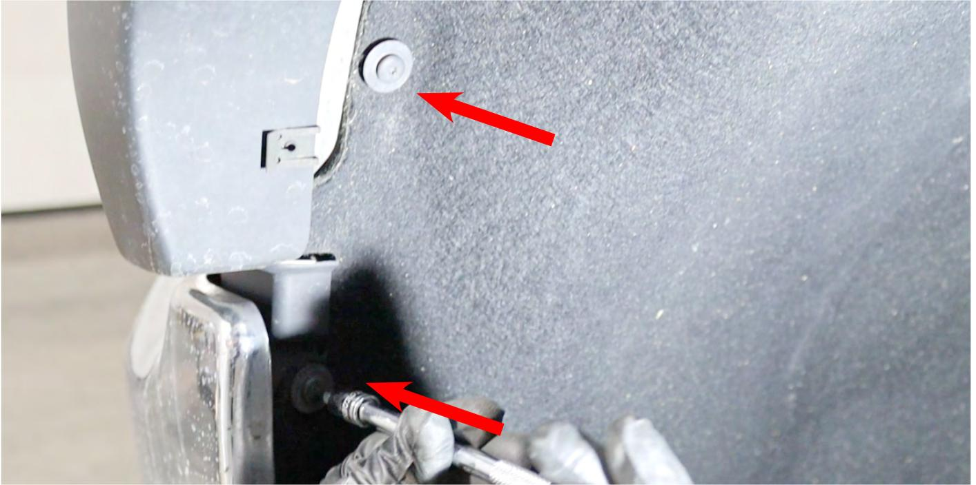
Subsequently, use a panel popper to widely open the guard cover, providing access to the headlight's bolt. Utilize a ratchet and extension socket to help remove the 10mm bolt. Repeat the same steps for the other side of the headlight.
