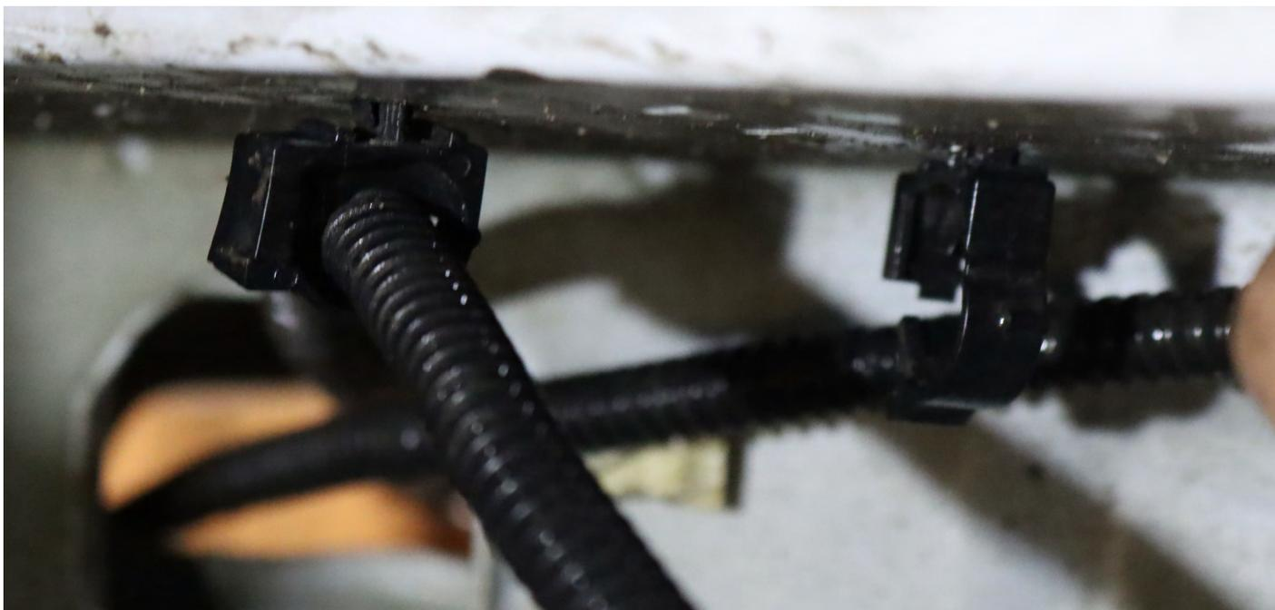
Once the tail lights and wirings are removed, please set them aside for the factory mounts transfer into your new ALPHAREX tail lights.
