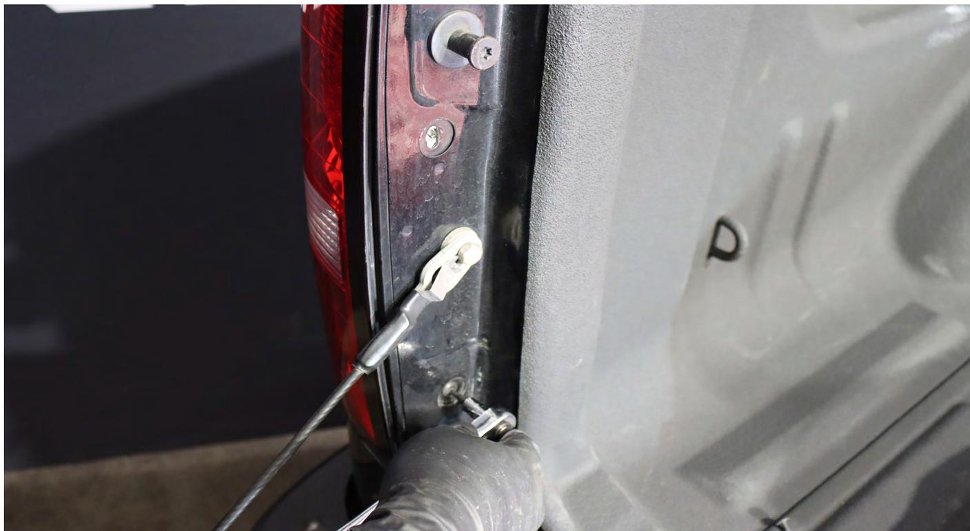
Take out the top and bottom T15 screws from each side of the tail lights.
