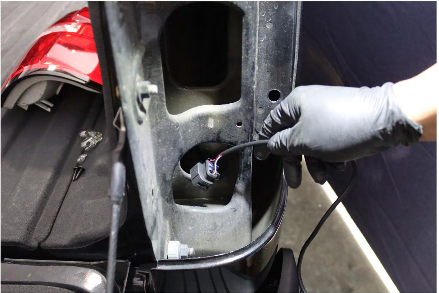
Route the tail light wiring into the truck as shown in the illustration, securing each section using the factory plastic connector mounts. **DO NOT USE DIELECTRIC GREASE!**
