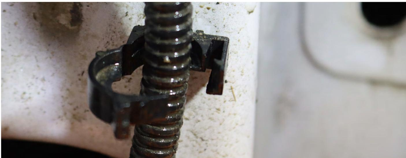
There are (2) cable clips securing the wiring for the driver's side tail light and (4) cable clips securing the wiring for the passenger's side tail light.
