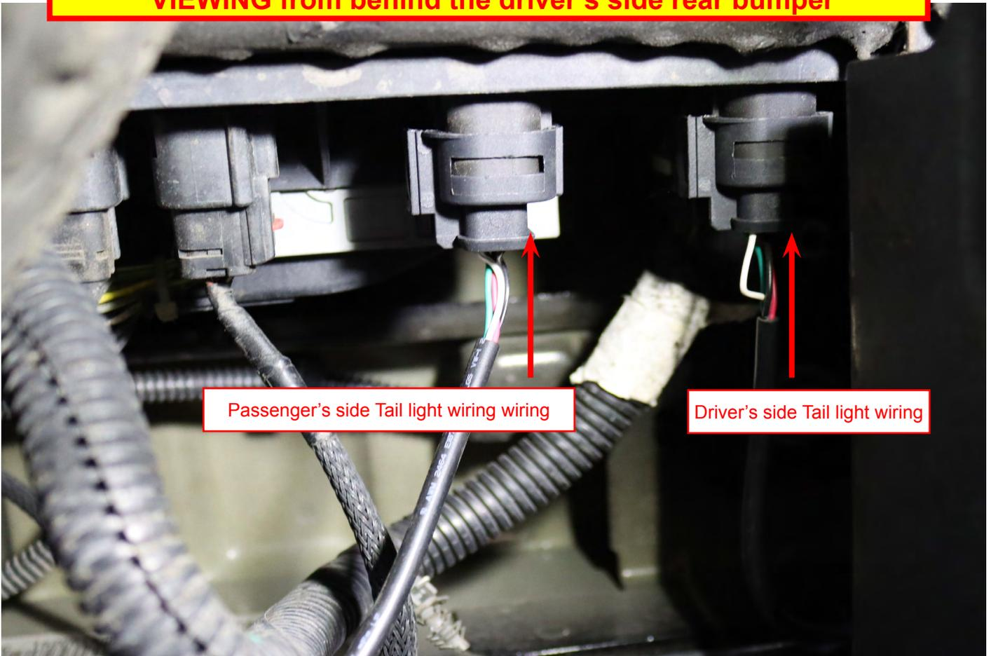
Passenger's side Tail light wiring
