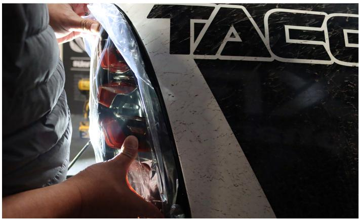
Use Phillips screw driver to tighten the 2 X 10mm screws for each side.
