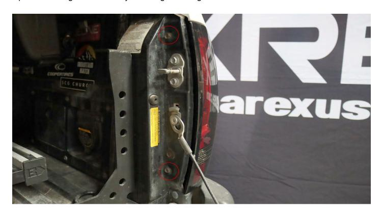
Remove the top and bottom 10mm screws from each side of the tail lights.
