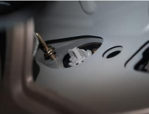
1.4 - With the bolts removed, you can now take out the tail light. There will be a single connector attaching it to the vehicle—disconnect it to fully release the light.
