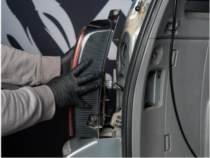
2.2 - Now, securely tighten the two 10mm bolts to hold the tail light in place.
